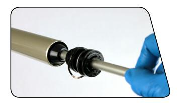
Install the snap ring onto internal snap ring pliers. Use the pliers to push the air shaft into the upper tube while installing the snap ring into its groove. The air shaft guide should be situated between the snap ring eyelets.
