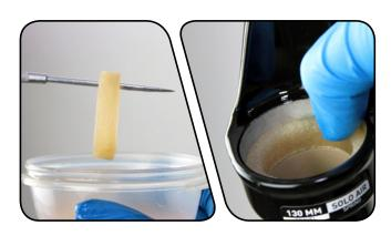
Use a seal installation tool to install the new dust wiper seals. Position the dust wiper into the recessed side of the tool, so the grooved side of the seal is visible.
