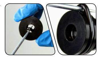
Use a pick to remove the air piston outer o-ring.
