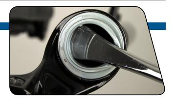
Stabilize the lower legs on a bench top or on the floor. Hold the lower legs firmly and use downward force on the tool handle to leverage the dust wiper seal out. Repeat on the other side.
