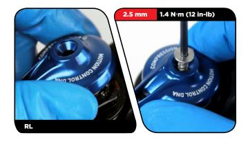
**Remote Only:** Install the cable stop collar onto the top cap with the cable stop facing toward the front of the fork, perpendicular to the crown. Use a 2 mm hex bit socket to tighten the collar clamp bolt to 1.4 N·m (12 in-lb).
