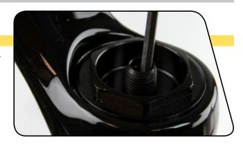
Use a 24 mm socket wrench to remove the air spring top cap. Once removed, clean the upper tube threads with a rag.
