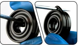
Spray isopropyl alcohol on the rebound damper shaft and clean it with a rag.
