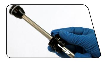
Use a pick to remove the inner and outer floating seal head o-rings. Inspect the seal head for scratches. Spray isopropyl alcohol on the seal head and clean it with a rag.
