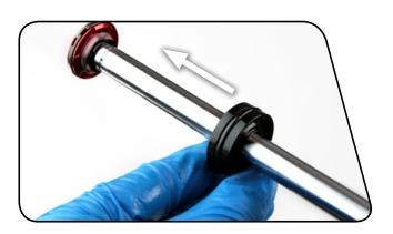
Insert the rebound damper piston into the bottom of the upper tube at an angle with the side opposite the glide ring split entering first. Continue to angle and rotate until the glide ring is in the upper tube.
