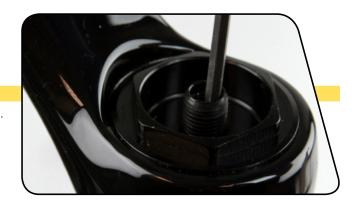
Remove the external rebound adjuster knob by pulling it from the shaft bolt at the bottom of the drive side fork leg.
