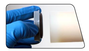
Hold one of the lower legs and use the seal installation tool to push the dust wiper seal evenly into the lower legs until there is no gap between the dust wiper seal and lower legs.
