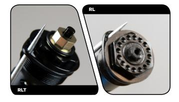
Use a pick or your fingers to remove the compression damper piston o-ring. Apply suspension fluid to the new o-ring and install it.
