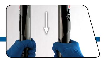
Spray isopropyl alcohol on the inside and outside of the lower leg. Wipe the outside of the lower leg with a rag.
