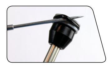
Use your fingers to remove the bumper cone from the air shaft. Install a new bumper cone onto the air shaft so it covers the tension pin hole.
