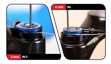
Disconnect the cable from the damper and pull the cable housing off the cable.
