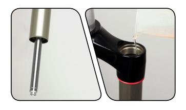
Turn the hex shaft to the unlocked position. Insert the compression damper into the upper tube. Press down and rock side to side until the damper is installed.
