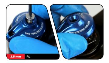
**Remote Only:** Use a 2 mm hex wrench to loosen the cable pinch bolt and remove the cable.
