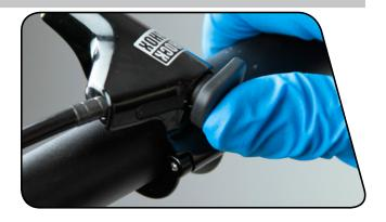
**RLT:** Use a 2 mm hex wrench to loosen the cable pinch bolt on the spool and pull the cable out of the cable end slot. Use pliers to remove the cable end.
