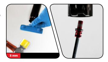
6 Firmly pull the lower legs downward until fluid begins to drain. Remove the lower leg from the fork by pulling it downward, holding onto both legs or the brake arch.
