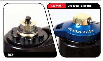
**RL:** Install the compression adjuster knob with the knob dial against the hard stop.
