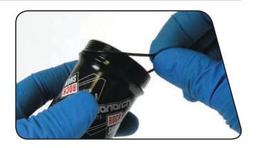
2 Use a pick to pierce the air can dust wiper seal and o-ring located inside the dust wiper seal gland. Push or pull to remove them, paying attention to the orientation of the dust wiper seal for reinstallation.
