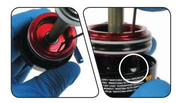
Spray the entire shaft and piston assembly with isopropyl alcohol and wipe it with a clean rag.
