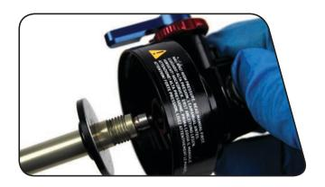
Use the SRAM shaft clamp tool to clamp the seal head/air piston into a vise with the eyelet positioned vertically.
