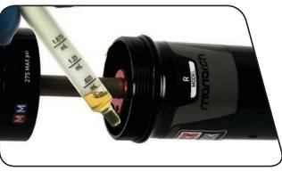
4 Continue to press the air can onto the damper body until the air can threads and shaft eyelet threads make contact. Thread the air can clockwise into the shaft eyelet. Tighten the air can, by hand, into the shaft eyelet.
