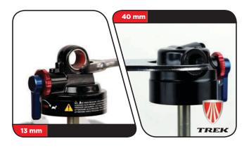
Remove the shaft assembly from the vise. Unthread the shaft from the eyelet by hand.
