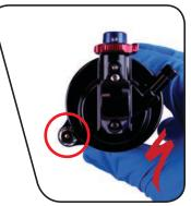
Use a Schrader valve tool to install a new Schrader valve into the air can valve.
