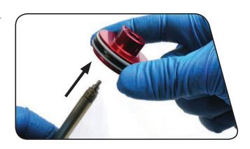
Use a pick to remove the o-ring located in the interior of the seal head.
