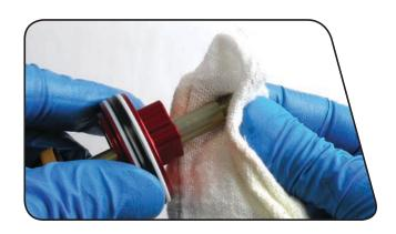
12 Install the bottom out o-ring and washer onto the shaft.
