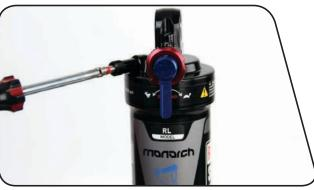
Use a Schrader valve tool to remove the air/nitrogen port cap.
