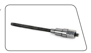
Insert the threaded rod through the shaft eyelet until the push pin rests against the bushing pin.
