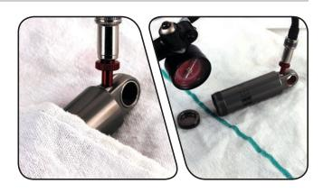
2 Spray isopropyl alcohol on the inside and outside of the damper body and wipe it with a clean rag.
