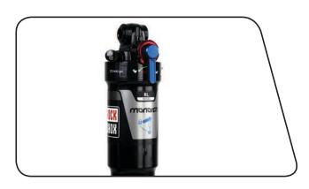
**6** Stabilize the air can with a strap wrench to prevent it from rotating. Use a torque wrench with a 13 mm (Trek®: 40mm) crowfoot socket to tighten the air can to 17 N·m (150 in-lb).
