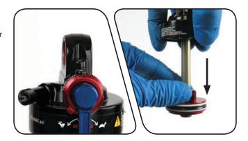
5 Install the seal head/air piston onto the damper body and thread it completely onto the damper body.
