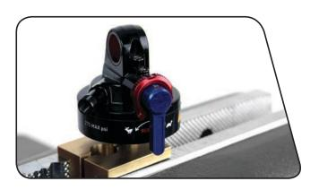
Use a 13 mm (Trek®: 40 mm) open end wrench to loosen the eyelet.
