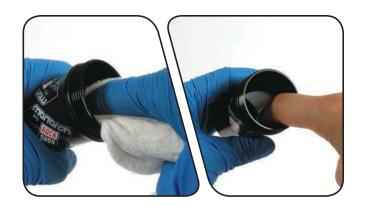
Install the new step bushing ring, quad ring, back-up ring, and dust wiper seal.
