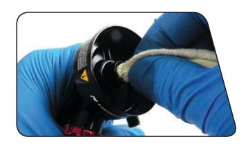
Turn the rebound adjuster counter-clockwise until it stops.
